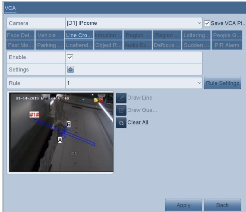
Figure 9. 6 Draw Line for Line Crossing Detection
