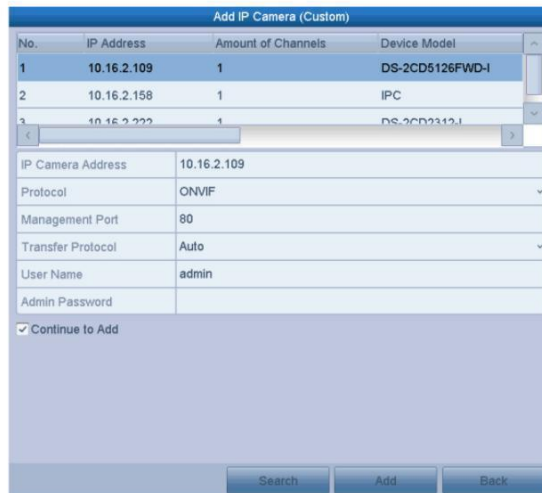
Figuur 2. 20 Custom Adding IP Camera Interface
